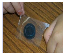
Fig. 4. Liquid crystal paint maps temperature of a hand
