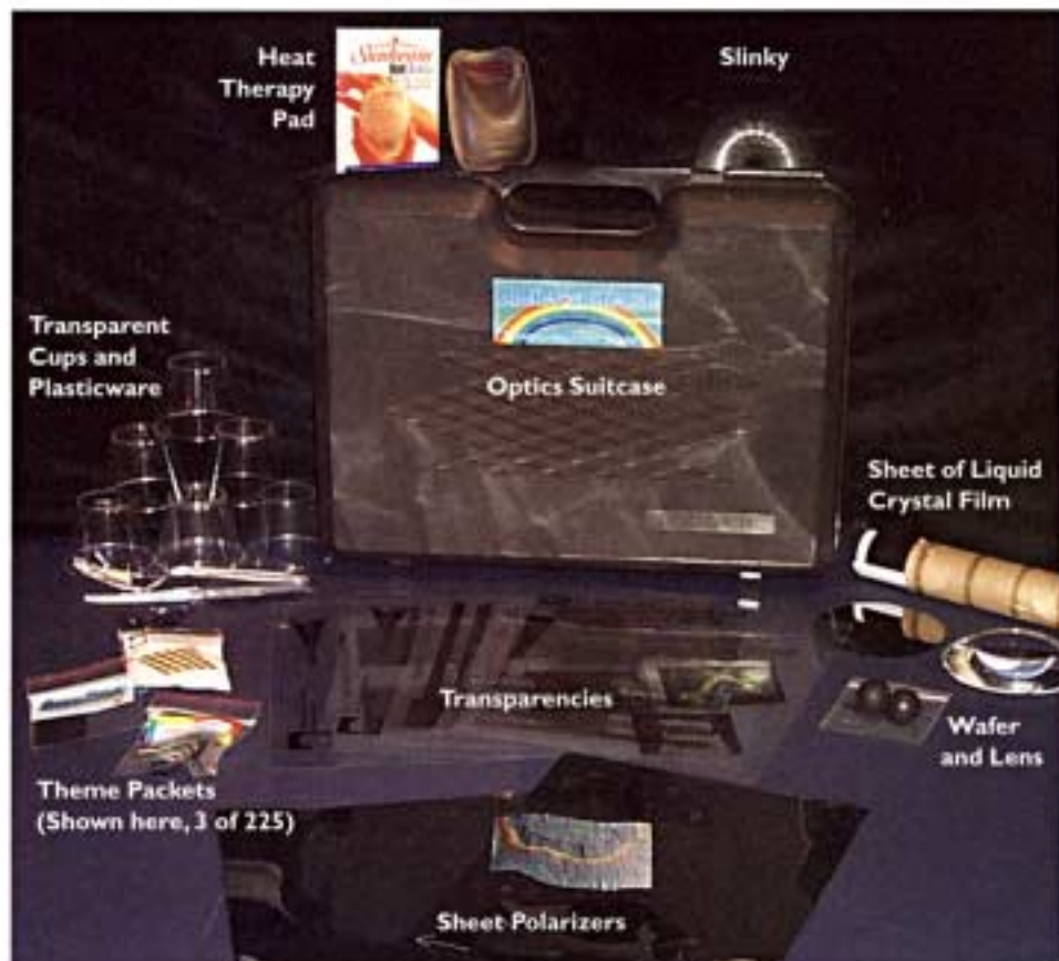
Figure 1. What's in the suitcase? Experiments to teach children about color by diffraction, color by polarization, color by selective reflection, and much more.
